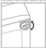
1. Install the washing machine on a flat sturdy floor, without resting it up against walls, furniture cabinets or other. 2. If the floor is not perfectly level, compensate for any unevenness by tightening or loosening the adjustable front feet (see figure); the angle of inclination, measured according to the worktop, must not exceed 2°.
